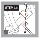
Slide Gas Tank Caddy under Cart, so top bracket piece rests on cart frame and is lined up with bolt hole on bottom of Gas Tank Caddy.
