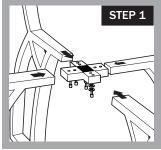
connector. Screw in casters and tighten nuts using wrench provided. While assembling, leave screws loose to allow adjustment in cart. Otherwise it can be difficult to get all of the screws in. After cart is assembled, confirm all bolts are tightened, then lift Kamado and set into cart with bottom vent centered between two legs.
