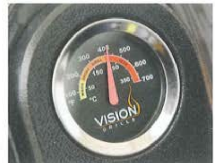
On the thermometer the temperature is indicated in the units of measure • c and ° F. By grouping in different temperature zones, it is directly apparent to which purpose which temperatures are recommended.
